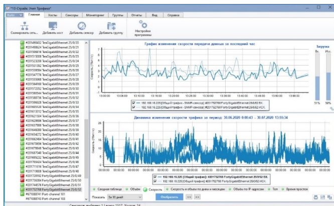
Fig. 6. I/O interfaces load between the links of the distribution level and the access level.
